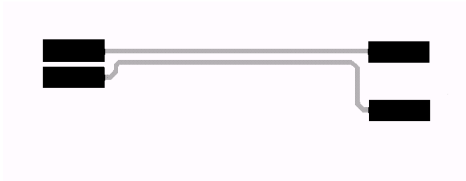
Figure 1. Correct MDI Trace Routing
