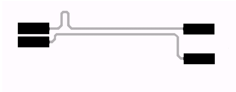
Figure 2. Incorrect MDI Trace Routing
