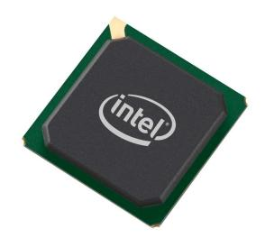
Intel® 82580 supports the MDI (Copper) standard IEEE 802.3 Ethernet interface for 1000BASE-T, 100BASE-TX, 10BASE-T connections (802.3, 802.3u, 802.3ab), the SERDES interface for 1000Base-SX/LX optical fiber connections, the 1000BASE-KX and 1000BASE-BX for backplane connections, and supports the SGMII interface for SFP/external PHY connections.
