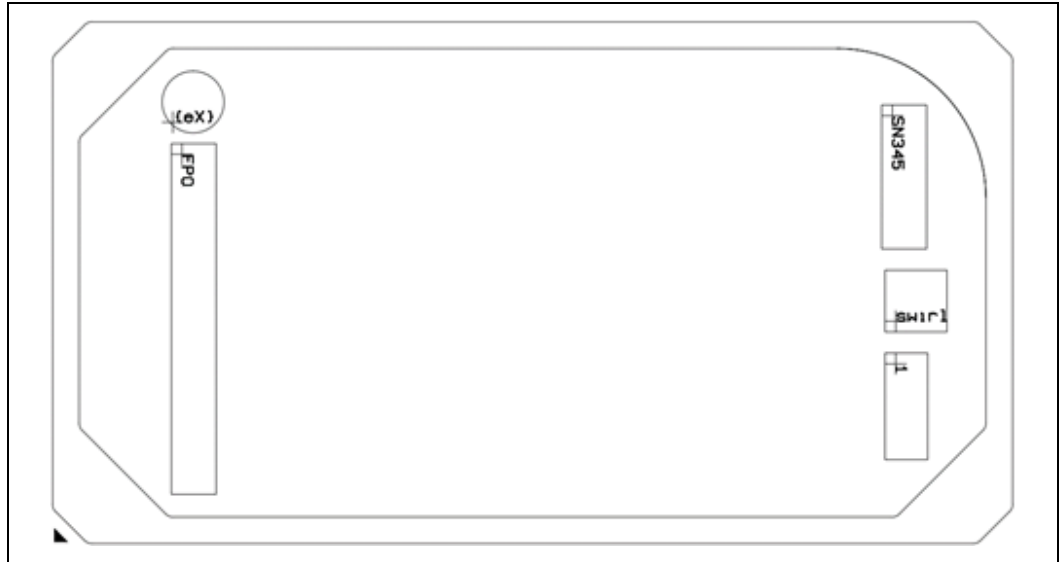
Figure 2-1. Based on UP3-Processor Line Multi-Chip Package BGA Top-Side Markings
