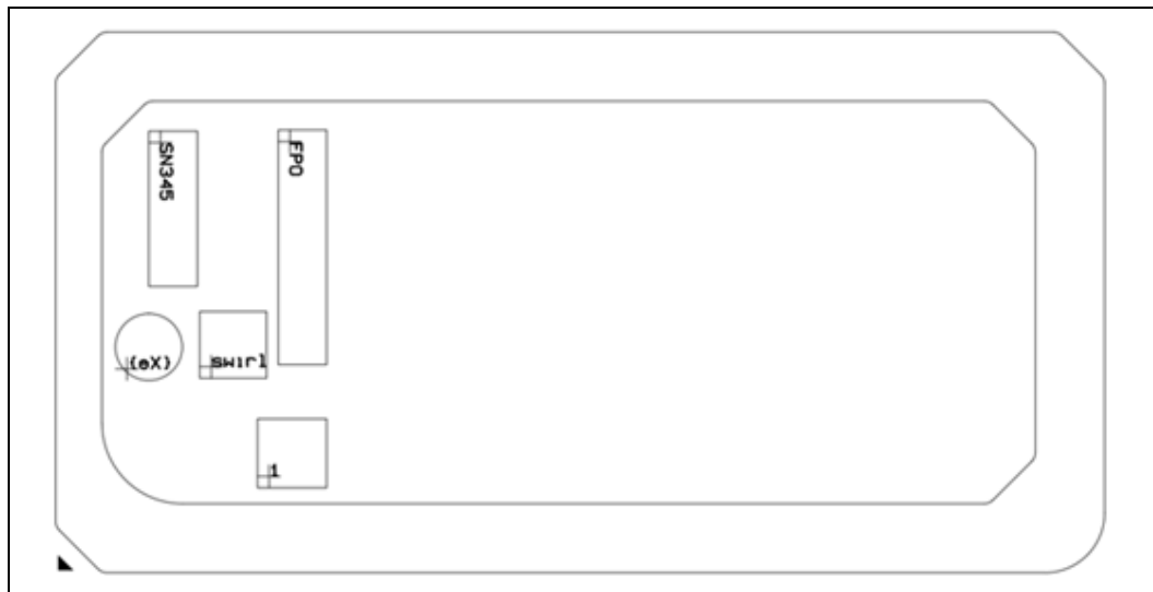
Figure 2-1. U-Processor Line Multi-Chip Package BGA Top-Side Markings
